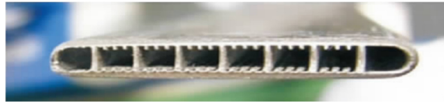
Fig 2. Cross section of micro heat pipe array
